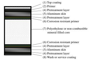
that the cut edge will be continuously exposed to moist conditions, a suitable corrosion protection will be necessary in the panel design or the fixing detail.
