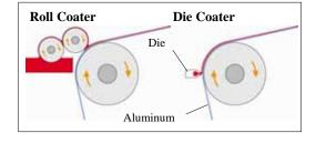
Fig. 1-7 Roll Coater and Die Coater
